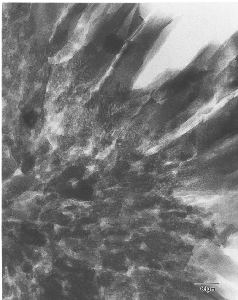
Figure 3--FeZSM-5 particle aggregate in as-synthesized form grown from an unstirred gel with \text{SiO}_2/\text{Fe}_2\text{O}_3 -ratio \approx 200 . The center of the FeZSM-5 particle (lower left area of the picture) consists of the small "hole" crystallites of FeZSM-5 and the outer edges are characterized by the larger FeZSM-5 crystals (upper right quadrant of the photograph).
