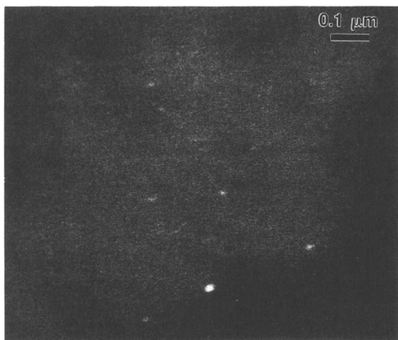
Figure 3. Platinum crystallites on a carbon film using axial dark field.
